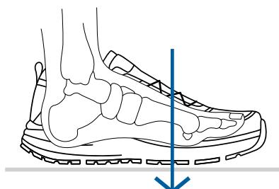
The back-shifted ball rocker facilitates the rolling off movement and reduces pressure in the forefoot area.
